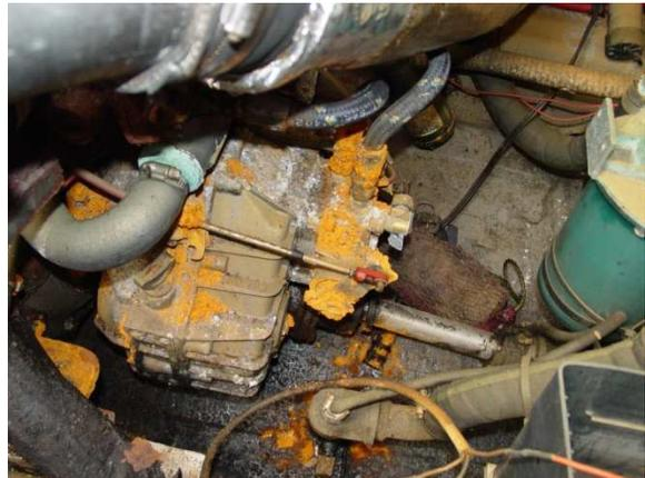
Photo 5: Example of engine corrosion
