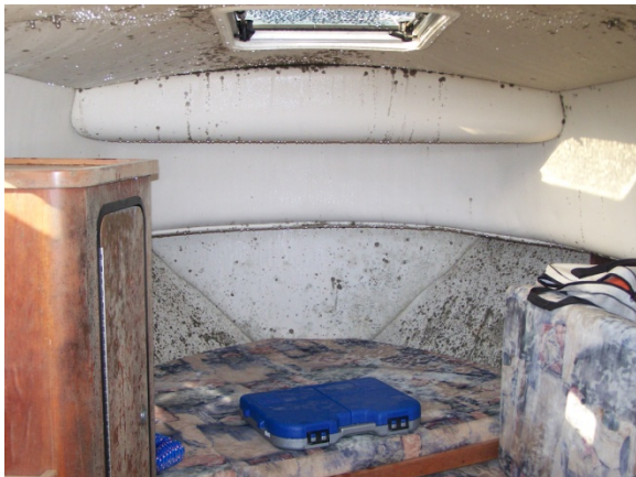
Photo 3: Mold and mildew in main cabin
